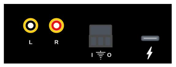
The digital contacts on the TX-device are used exclusively to implement relay control functionality.
