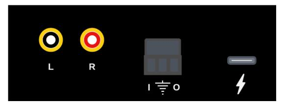
On the RX-device, the digital contacts are used to implement relay control functionality as well as for Factory reset.
